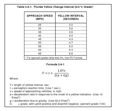
All of the variables in the equation have assumed or fixed values except the approach speed, v. As a result, the speed of vehicles as they approach an intersection is the critical input an engineer must consider when solving the formula for Y – an appropriate length in seconds for the yellow light.
