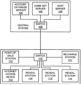
This diagram, from patent US 20070135209A1, illustrates a sweepstakes system. Each item can be a separate device, or multiple items can be within one device.
