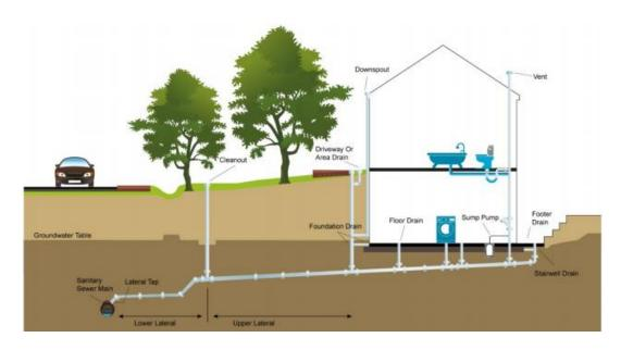
Sanitary sewer laterals are often in poor condition and defects can occur due to aging systems, structural failure, lack of maintenance, or poor construction and design practices.<sup>4</sup> Problems in
