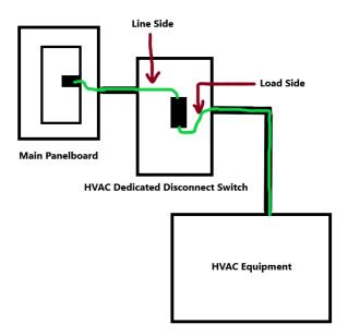
A dedicated circuit has its own circuit breaker and only supports one outlet, which means only one electrically powered device can draw voltage from that circuit at any given time.<sup>20</sup> A disconnect switch is used to isolate electrical circuits by interrupting the flow of electrical current. By quickly stopping the flow of power, disconnect switches allow for emergency shutdowns, switching to alternate power sources, and maintenance.<sup>21</sup>
