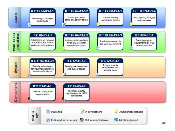
ISA 62443-1 defines the elements necessary to establish a cybersecurity management system for industrial automation and control systems (IACS) and provides guidance on how to develop those elements. It defines IACS as a "collection of processes, personnel, hardware, and software that can affect or influence the safe, secure, and reliable operation of an industrial process." ISA 62443-1 also lists the seven foundational requirements:
