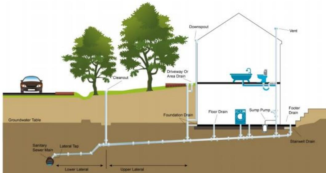
Sanitary sewer laterals are often in poor condition and defects can occur due to aging systems, structural failure, lack of maintenance, or poor construction and design practices.<sup>4</sup> Problems in
