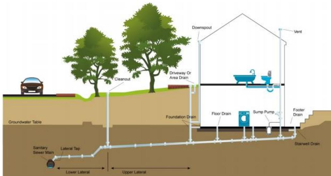
Sanitary sewer laterals are often in poor condition and defects can occur due to aging systems, structural failure, lack of maintenance, or poor construction and design practices.<sup>3</sup> Problems in sanitary sewer laterals can have a significant impact on the performance of the sewer system and treatment plant and can account for half of the infiltration and inflow to sanitary sewers.<sup>4</sup> Cracked or broken laterals can allow groundwater and infiltrating rainwater to enter into the
