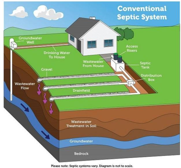
In a conventional OSTDS, the septic tank does not reduce nitrogen from raw sewage. Approximately 30-40 percent of the nitrogen levels are reduced in the drainfield of a system that is installed 24 inches or more from groundwater.<sup>21</sup> This still leaves a significant amount of nitrogen to percolate into the groundwater, which makes nitrogen from OSTDSs a potential contaminant in groundwater.<sup>22</sup>
