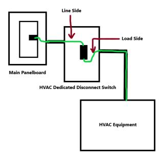
A dedicated circuit has its own circuit breaker and only supports one outlet, which means only one electrically powered device can draw voltage from that circuit at any given time. A disconnect switch is used to isolate electrical circuits by interrupting the flow of electrical current. By quickly stopping the flow of power, disconnect switches allow for emergency shutdowns, switching to alternate power sources, and maintenance.
