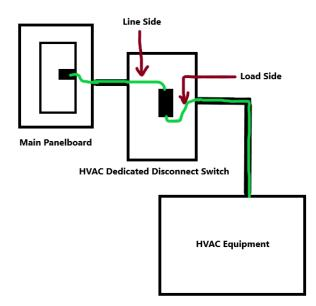
A dedicated circuit has its own circuit breaker and only supports one outlet, which means only one electrically powered device can draw voltage from that circuit at any given time.<sup>21</sup> A disconnect switch is used to isolate electrical circuits by interrupting the flow of electrical current. By quickly stopping the flow of power, disconnect switches allow for emergency shutdowns, switching to alternate power sources, and maintenance.<sup>22</sup>
