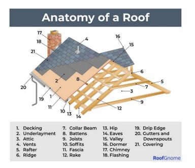
Roof sheathing, also called roof decking, are the wooden boards that make up the framing of a roof system. These boards are what shingles and other roofing components are installed directly on.<sup>12</sup>
