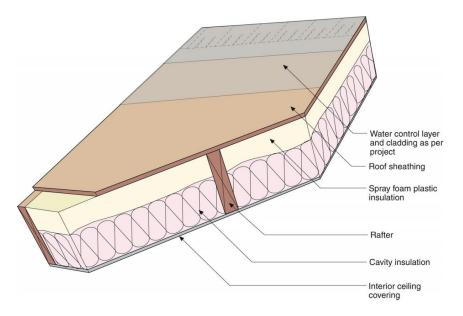
Florida generally requires insulation to be installed under the roof sheathing,<sup>22</sup> but elsewhere, airimpermeable insulating sheathing applied over the roof deck may be used for unvented attics, and is typically installed as follows:<sup>23</sup>
