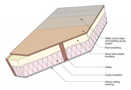
Florida generally requires insulation to be installed under the roof sheathing, 65 but elsewhere, air-impermeable insulating sheathing applied over the roof deck may be used for unvented attics, and is typically installed as follows: 66
