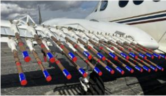
Wing-Mounted Burn-In-Place Flares 16
